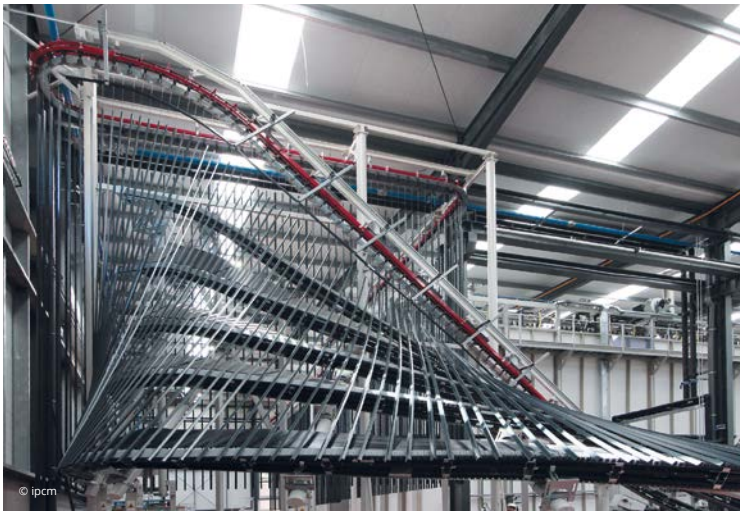
From top left clockwise: Powder application with Gema SIT technology; The powder centres of the two C-Expert booths; The automatic unloading system with five transport belts; Storage buffers housing the coated profiles to be sorted towards the assembly, packaging, and plasticisation lines.
