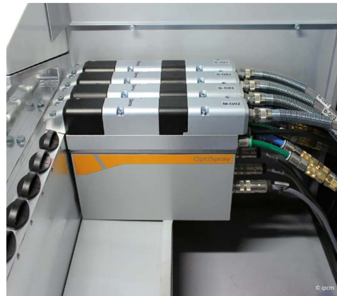
Workpieces leaving the coating booth and the OptiSpray AP 01 feed pumps with Smart Inline Technology.
