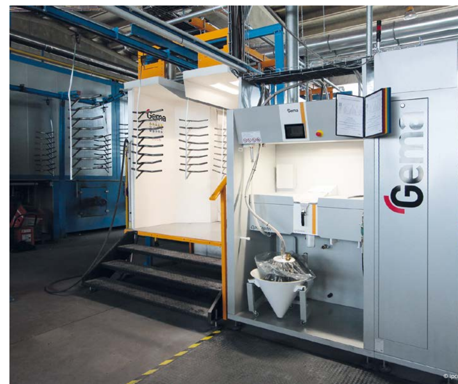
Gema's MagicCompact automatic booth and OC07 powder management unit.
