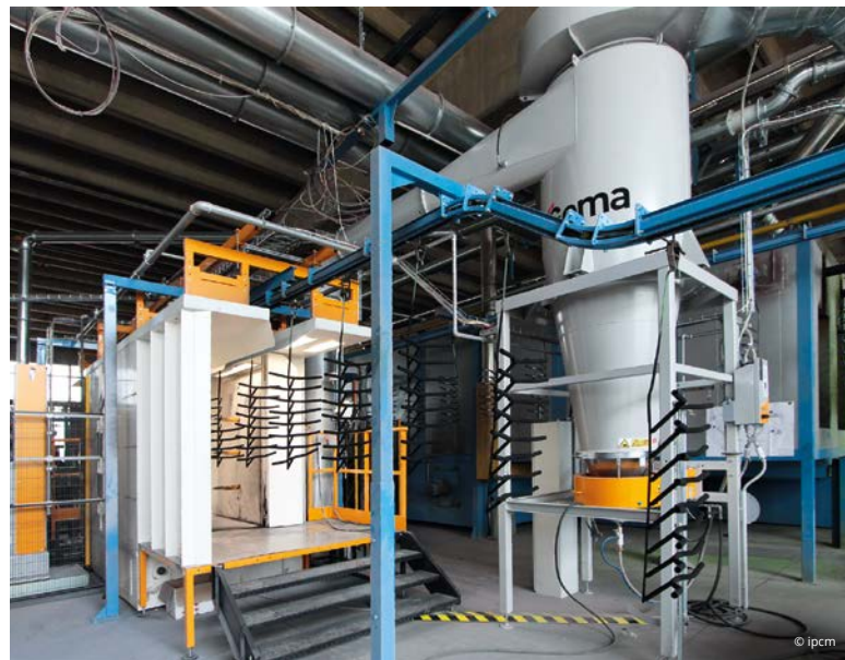
Workpieces leaving the coating booth and the OptiSpray AP 01 feed pumps with Smart Inline Technology.
