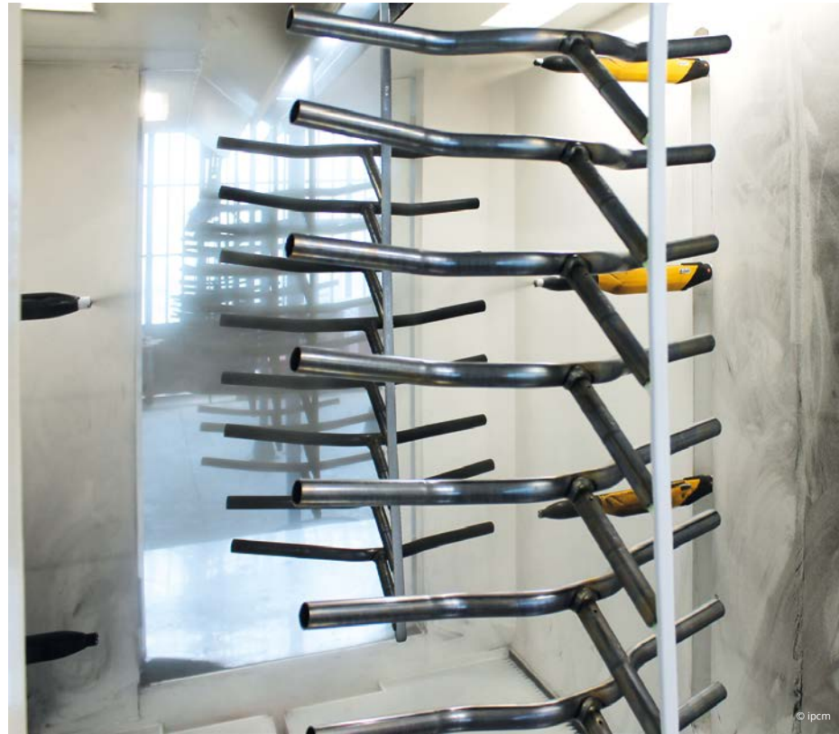
Sa.Ve.M. parts at the entrance to the coating booth.
