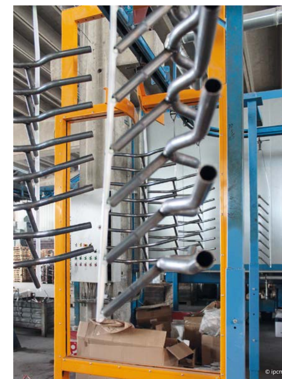
Bicycle handlebars moved from the overhead conveyor to the chemical pre-treatment tunnel.
